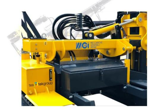
**CROSS COLUMN** - Contains the mechanism for the transverse movement of the column
