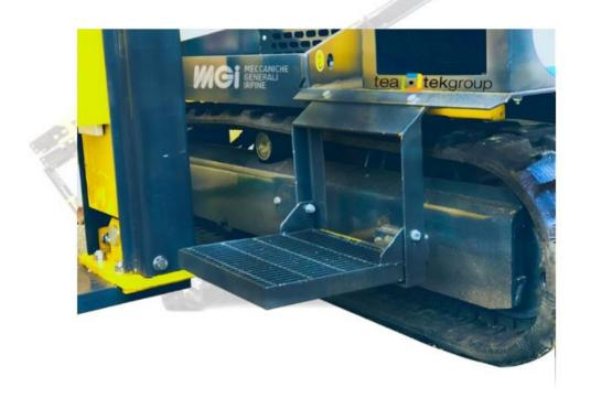
FOOTBOARD - Used by the operator to stand on when driving the machine with good standards of comfort and safety.
