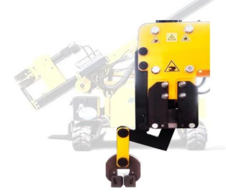
**STEEL POLE EXTRACTOR** - By means of this device it is possible to apply a force up to 6,000 kg in extraction tasks (Attachment available upon customer request, it is not included in the price of the machine).
