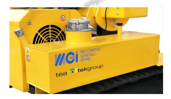
**FUEL & HYDRAULIC OIL TANKS -** These supply the internal combustion engine and the hydraulic system of the machine
