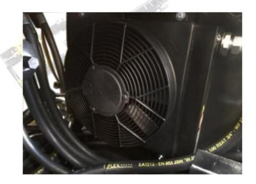
**HEAT EXCHANGER-** It dissipates the excessive heat of the hydraulic oil.
