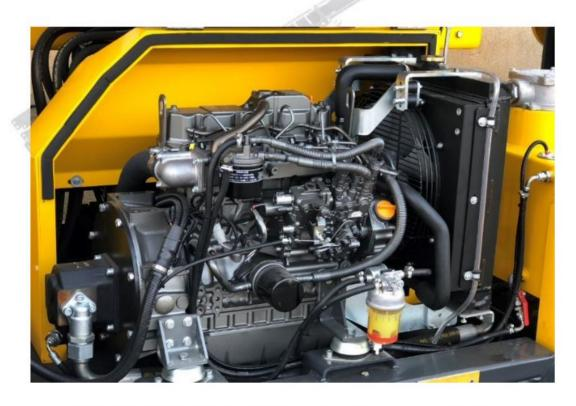
**INTERNAL COMBUSTION ENGINE** - It supplies energy to the hydraulic components of the machine
