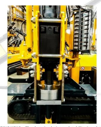
**SWINGING HEAD** – Thanks to its design and stability, it makes possible the rapid insertion of wood /steel piles, having different cross-sections up to a size of 300 mm. The design, choice of material and shape of each head, can be made according to the customer's requests
