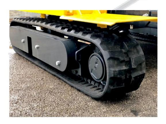
**CRAWLER CART** – The crawler cart dimensions are relevant. The specifications, being 2000 mm in length, 1980 mm in width and 480 mm in height, make it fast and highly manoeuvrable, even on uneven and rough ground.
